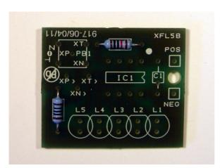
3. Insert the chip socket in the area marked IC1. Don't confuse this with the chip – the chip socket has eight little holes on top that the chip can be pushed into later. The notched end should be at the end marked with a notch on the board. Hold it fully in place and bend over a couple of the legs to hold it securely. Solder all the legs.
