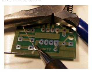
2. Apply Solder - make sure it flows both onto the pad and up the component leg, as here.
