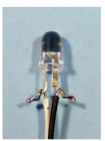
7. Cut the length of heatshrink tubing into five pieces. Heatshrink was not provided in 2010 edition kits - you can use sticky tape instead. Place a piece over the negative (black) wire of each LED and push right up against the LED. Shrink the tubing by holding it as near to the soldering iron as you can without touching it - about half an inch up from the tip works best. If you do touch the heatshrink with the iron, wipe off any molten plastic as soon as possible on the brass tip cleaner.
