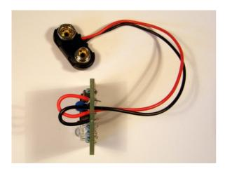
8. The chip pushes into the socket - the notched end MUST be nearest the capacitor.
