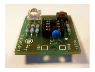
7. The battery lead goes up through the large hole from underneath the board, and then the leads bend over to the small holes, red to POS and black to NEG. Pull the leads tight enough that the ends stay in the holes. Solder the leads (tricky! Try using something heavy to hold the board down) then cut the ends off close to the board and pull the lead tight.
