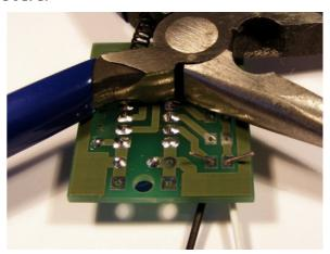
9. The battery lead goes up through the large hole from underneath the board, and then the leads bend over to the small holes, red to POS and black to NEG. Pull the leads tight enough that the ends stay in the holes. Solder the leads then cut the ends off close to the board and pull the lead tight.
