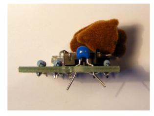
7. The Light Dependent Resistor (LDR) goes in the hole marked LDR. 2010 edition candles don't have an LDR.
