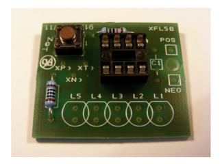
5. The capacitor (marked 104) goes in C1, either way round. There is a choice of two holes for the leg nearer the bottom of the board, depending on the size of capacitor in your kit. Hold it in place and bend the legs outwards, then solder. Cut the legs off as close to the board as you can.
