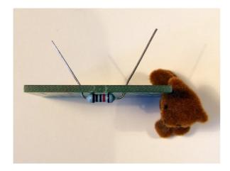
2. R2 is the 100R resistor (brown, black, black, black, brown). It can go either way round. Insert and solder as for the first resistor.
