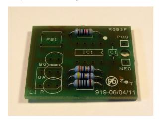
3. Insert the chip socket in the area marked IC1. Don't confuse this with the chip – the chip socket has eight little holes on top that the chip can be pushed into later. The notched end should be at the end marked with a notch on the board. Hold it fully in place and bend over a couple of the legs to hold it securely. Solder all the legs.
