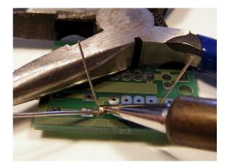
3. Stop applying solder - keep the iron on for another second or so.
